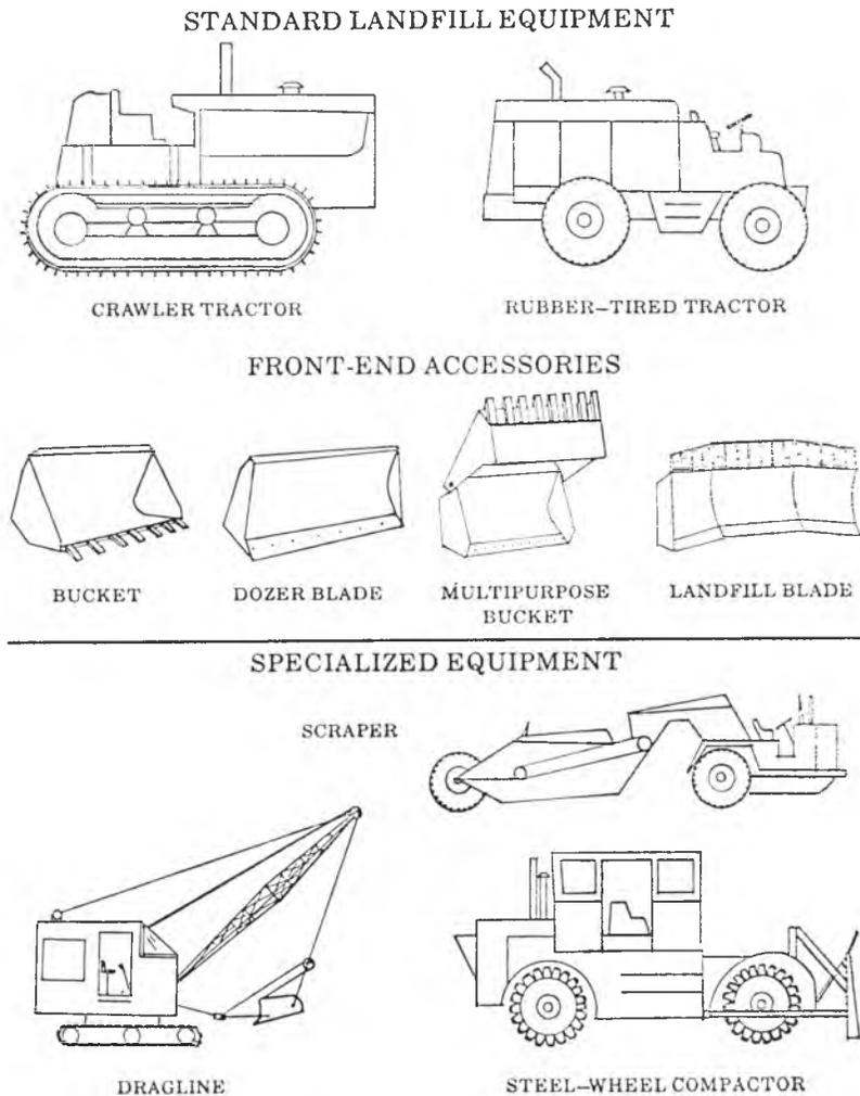
**Fig. 5. Standard and Specialized Landfill Equipment.**
