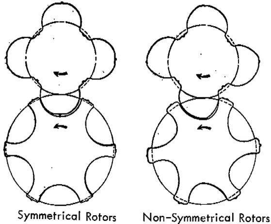
This improved performance is due to the reduction in size of the leakage triangle between the male and female rotor as shown in the photo below.
