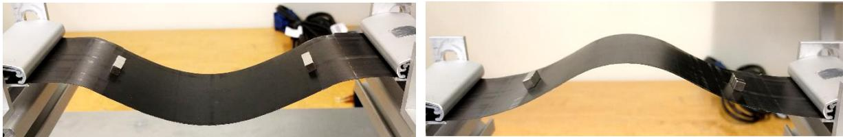
Figure 2. (a) Clamped-clamped laminate positioned at state 1 (low) with mass on the sides to aid in inducing larger oscillations. (b) Laminate positioned at state 2 (high).
