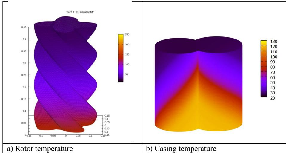
**Figure 6:** Assumed rotor and casing temperature distributions
