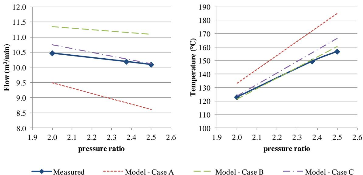
**Figure 10:** Compressor performance from test and model
