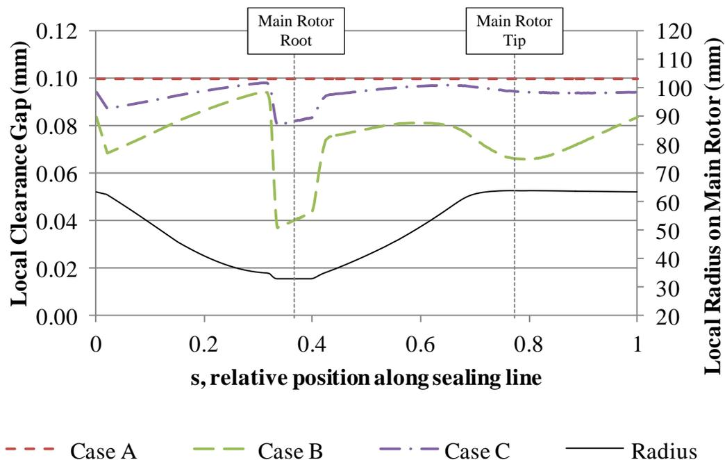
**Figure 8:** Interlobe clearance distribution corrected for thermal deformations
