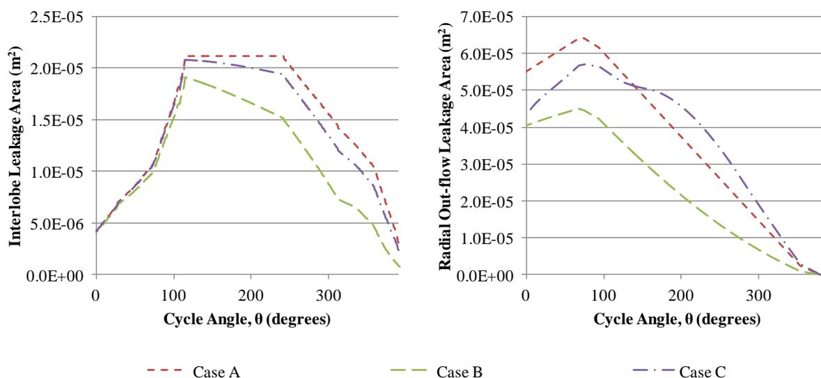
**Figure 9:** Variation of leakage areas throughout compression cycle
