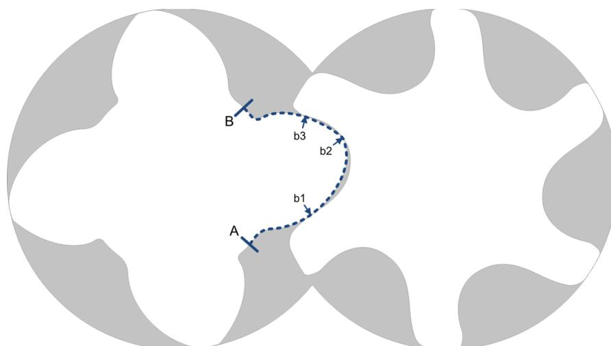
**Figure 3:** Identifying chamber boundaries on main rotor
