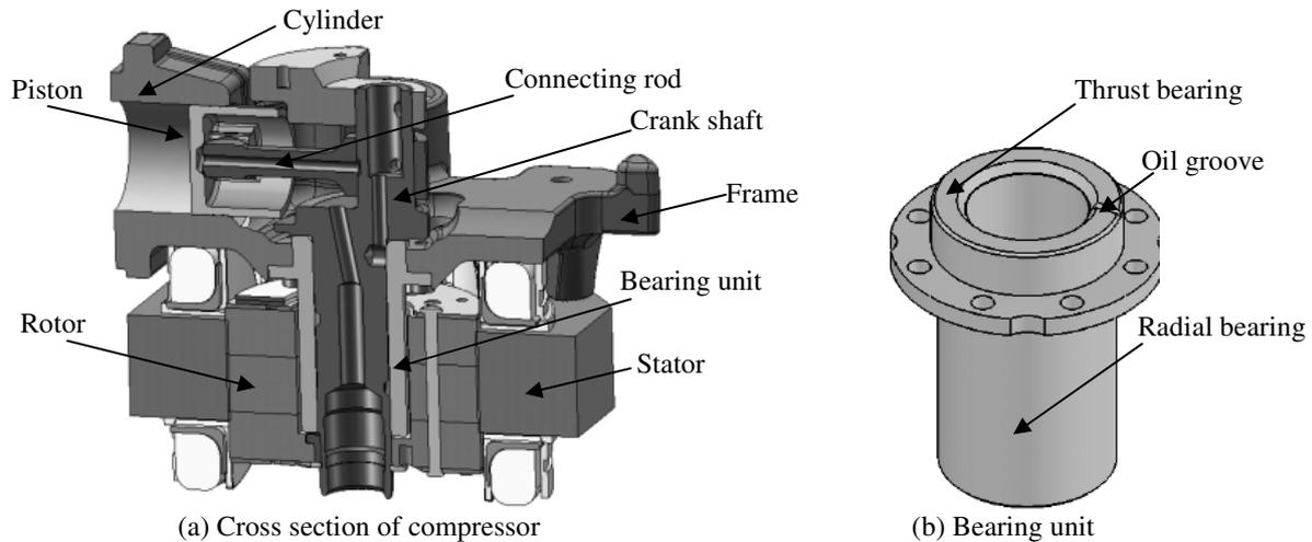
Figure 1: Experimental compressor
