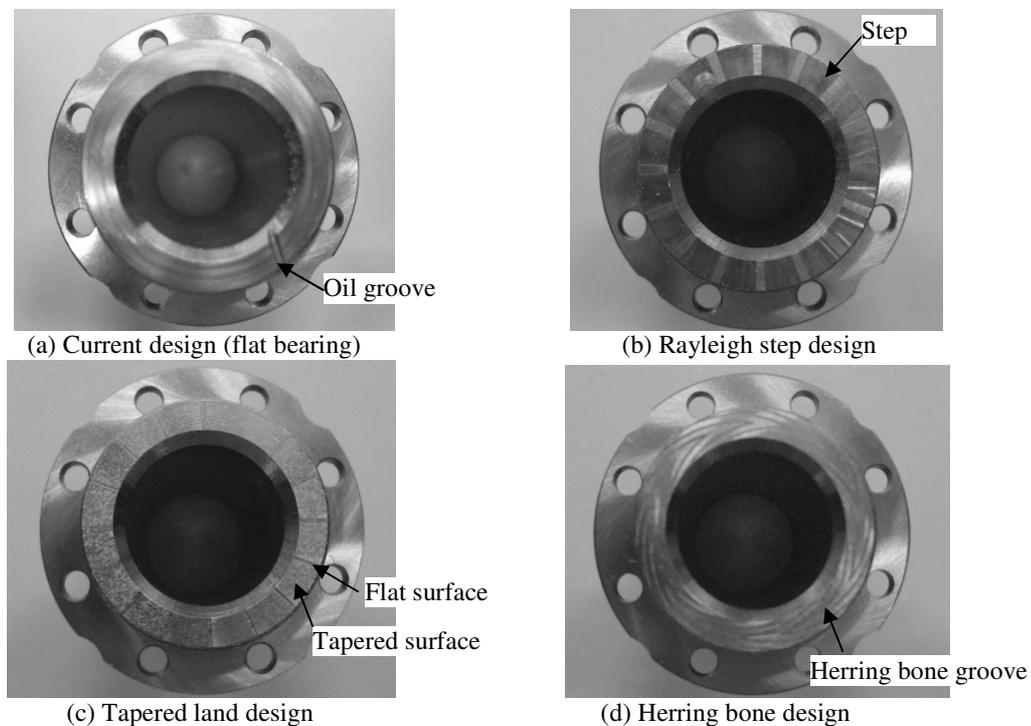
Figure 2: Thrust bearing test pieces (bearing units)
