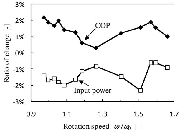
Figure 5: Improvement in efficiency with herring-bone-design thrust bearing
