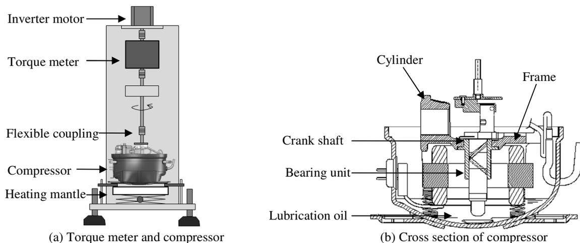
Figure 3: Schematics of apparatus for measuring friction torque of crank shaft
