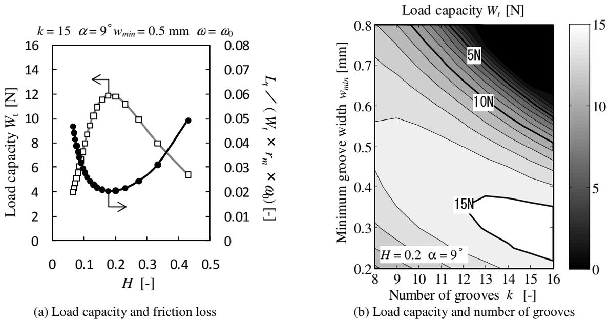
Figure 8: Properties of bearing with herring bone grooves
