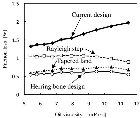
Figure 4: Friction loss of thrust bearings in elemental friction test
