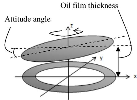
(b) Model of flat thrust bearing
