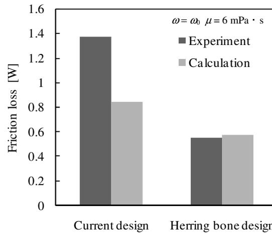
Figure 9: Comparison of experiment and calculation
