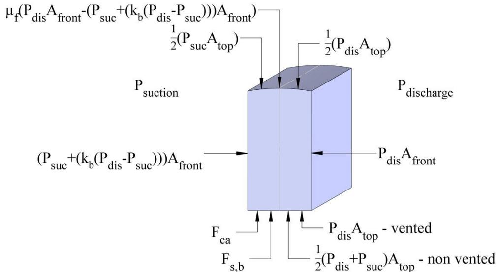
Figure 5: Static free-body diagram of tip seal forces.
