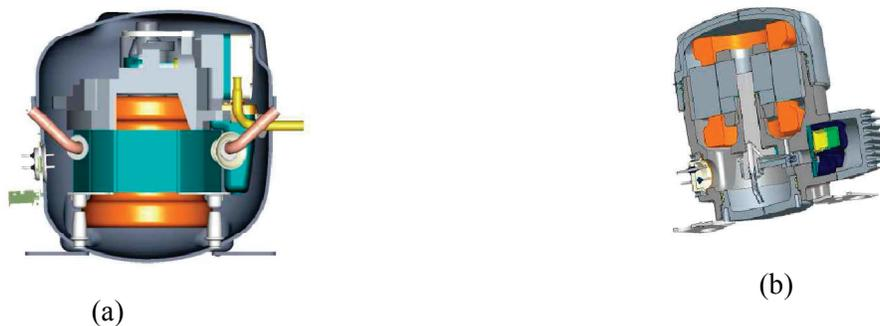
Figure 2: HFC compressor (a) present expressive differences when compared to CO<sub>2</sub> compressor.
