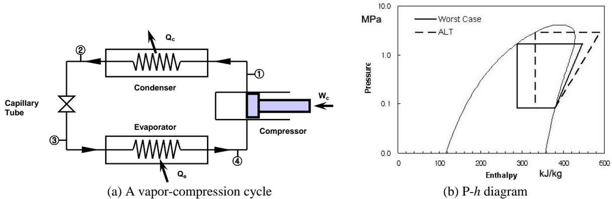
Figure 1: Schematic diagram for a vapor compression system
