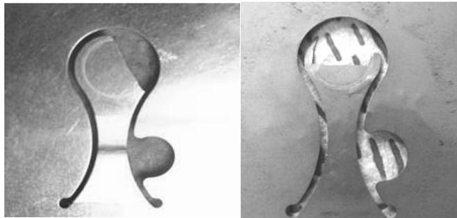
Figure 4: Failure of suction reed valve in marketplace
