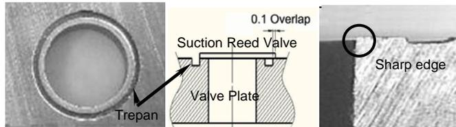
Figure 6: Structure of suction reed and valve plate
