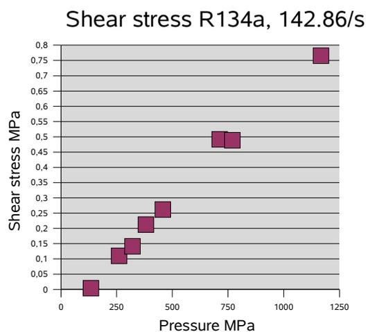
Figure 12. Shear stress for R134a at 142.86 s<sup>-1</sup>.
