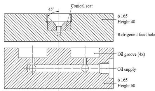
Figure 2. Hydrostatic bearing.
