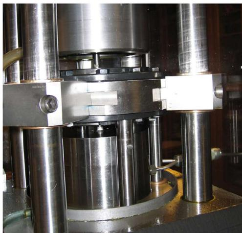
Figure 1. High pressure chamber and hydrostatic bearing.
