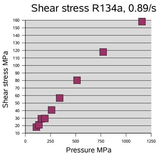
Figure 10. Shear stress for R134a at 0.89 s<sup>-1</sup>.
