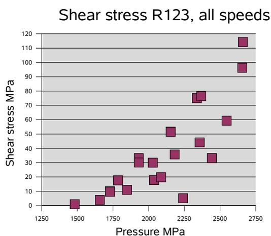
Figure 15. Shear stress R123 at all speeds between 0.89 and 142.86 s<sup>-1</sup>.
