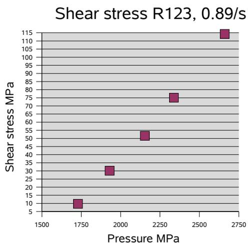
Figure 14. Shear stress for R123 at 0.89 s<sup>-1</sup>.
