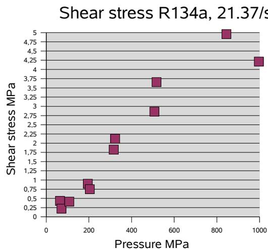
Figure 11. Shear stress for R134a at 21.37 s<sup>-1</sup>.
