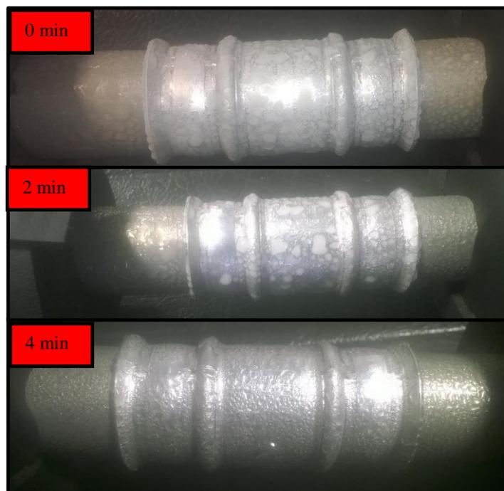
**Figure 11: Ice melting process during the thawing cycle of the 28.5 mm fitting**
