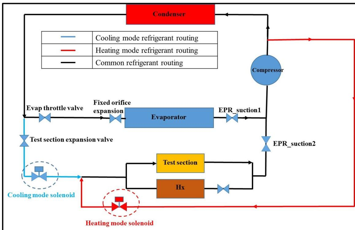
Figure 2: Facility schematic for heating and cooling mode
