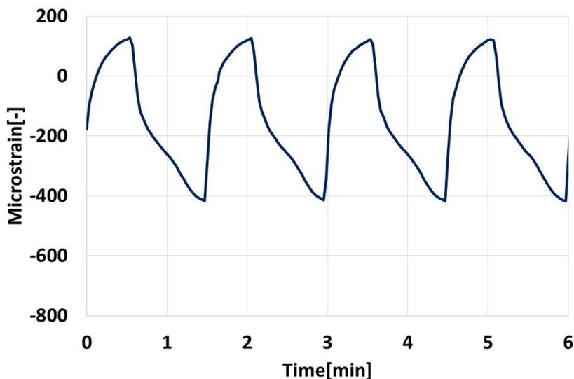
**Figure 4: Sample strain profile of a 28.5 mm fitting**
