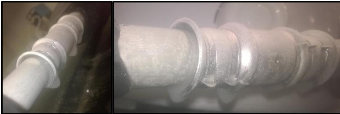
**Figure 10: Ice formation at the joints of the fittings**
