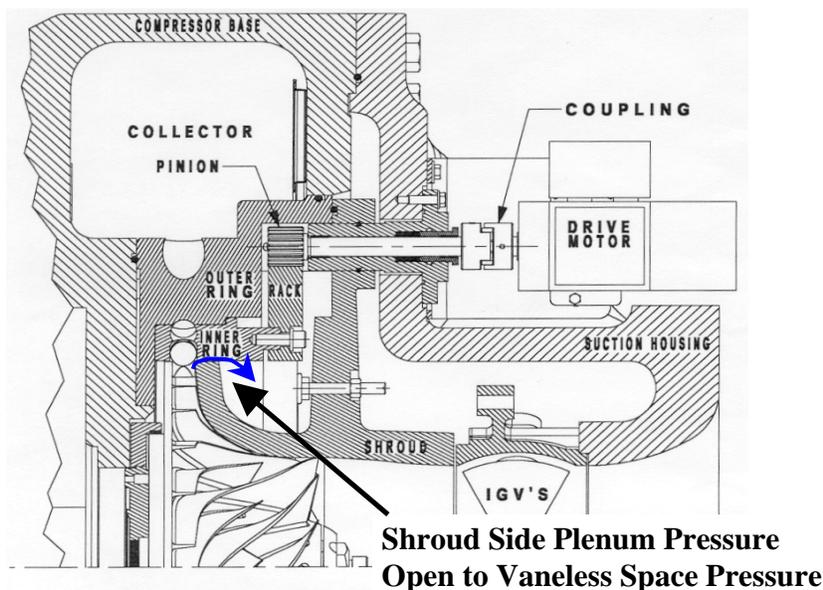
**Figure 1 Compressor Geometry**
