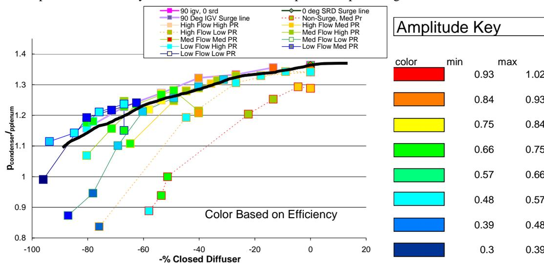
Figure 7 Diffuser Pressure Recovery Parameter Correlation to Variable Diffuser Orientation
