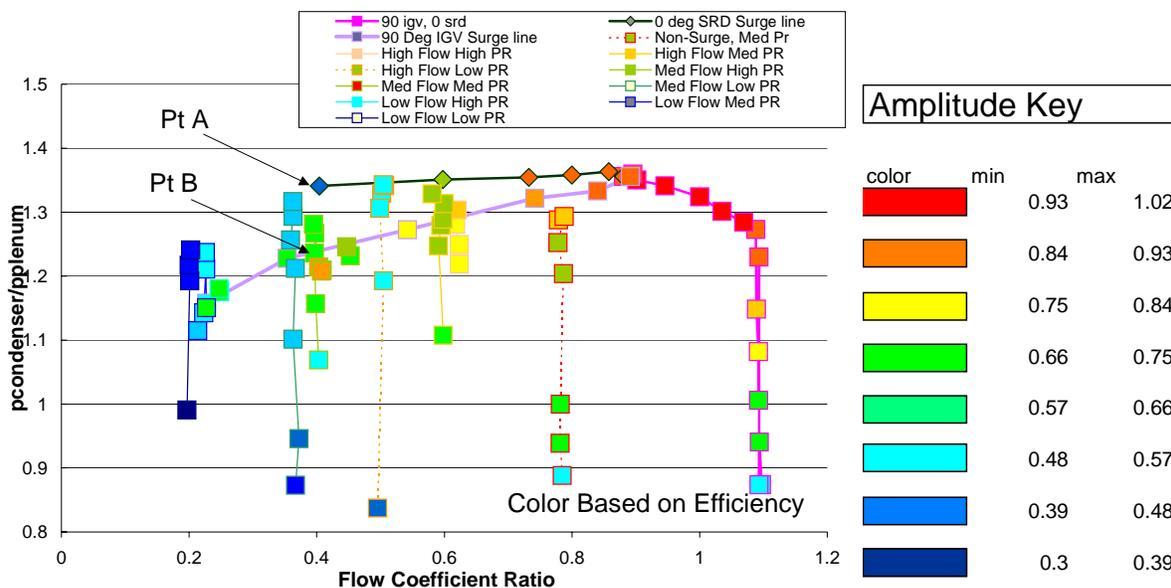
Figure 5 Diffuser Pressure Recovery Parameter Correlation to Efficiency
