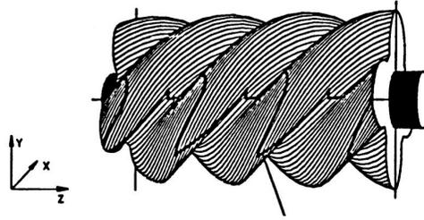
Fig. 2 Seal line on a male rotor (Diagram by courtesy of S. Jonsson (1985))
