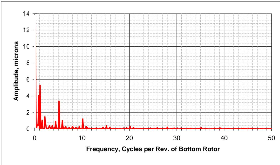
Fig. 5 Fourier Spectrum of Transmission Error
