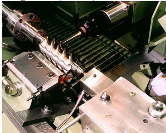
Fig. 1 Renishaw scanning probe on a Holroyd rotor grinding machine
