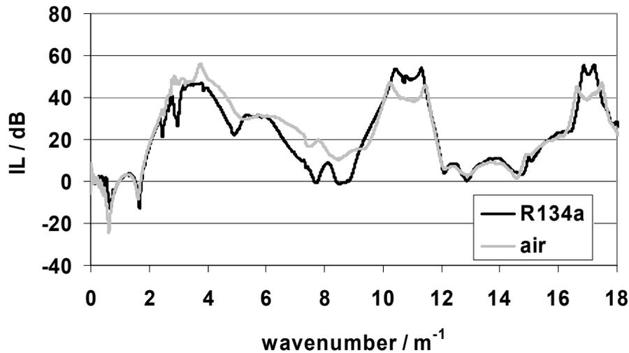
Figure 6: Comparison between measured IL in R134a and air.
