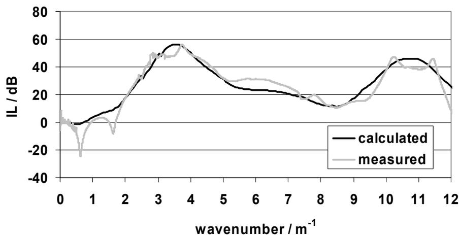
Figure 5: Comparison between calculated and measured IL.
