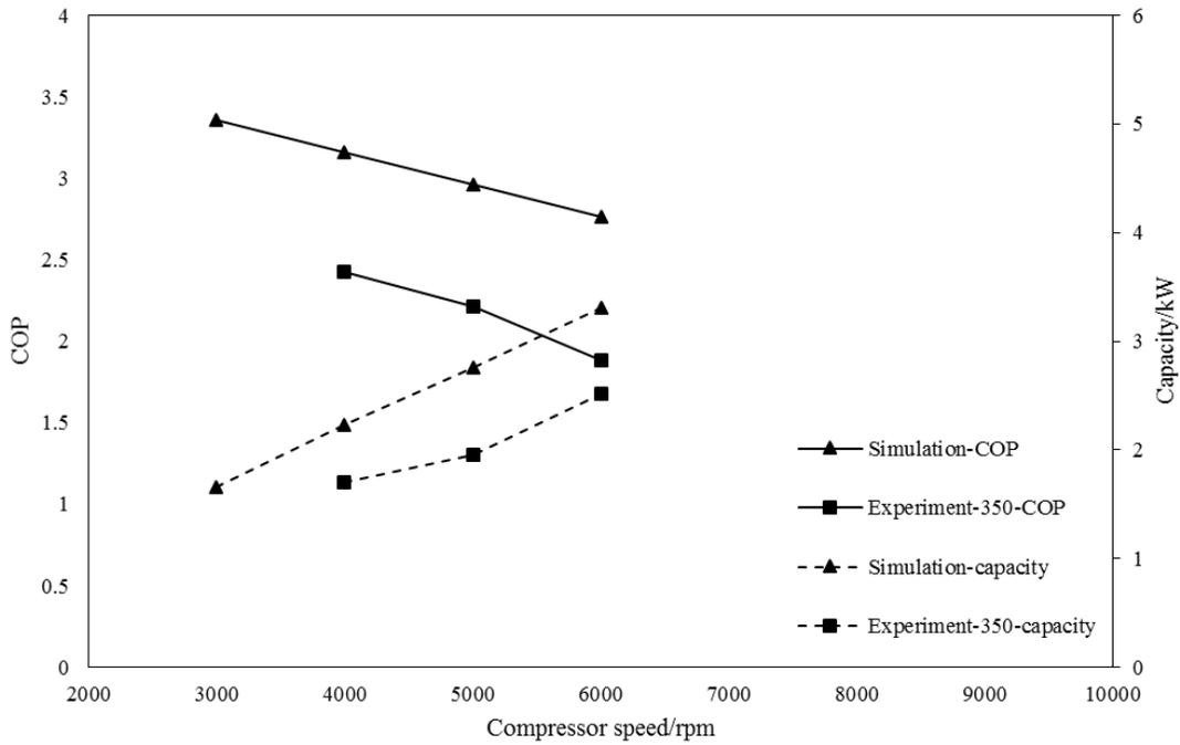
Fig 5: Simulation and experiment comparison of R407c system
