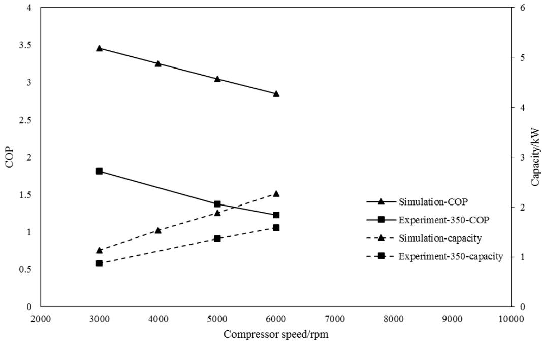
Fig 4: Simulation and experiment comparison of R134a system
