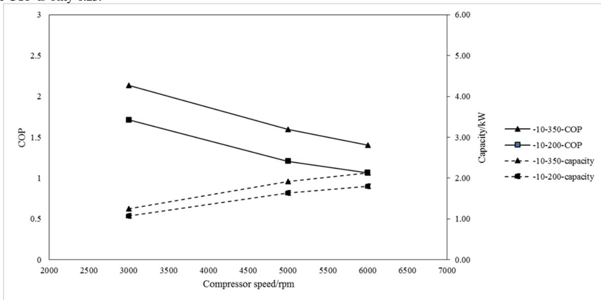
Fig 7: Effect of HVAC air flow rate
