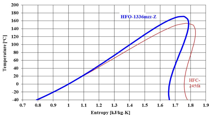
Figure 3: HFO-1336mzz-Z temperature-entropy diagram compared to HFC-245fa
