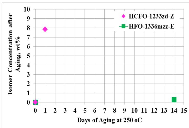
**Figure 5:** Concentrations (by GC-MS peak area) of HFO-1336mzz-E or HCFO-1233zd-Z in glass test tubes originally containing neat HFO-1336mzz-Z or HCFO-1233zd-E, respectively, after aging at 250 °C in the presence of carbon steel, copper and aluminum coupons
