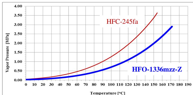
Figure 2: HFO-1336mzz-Z vapor pressure compared to HFC-245fa
