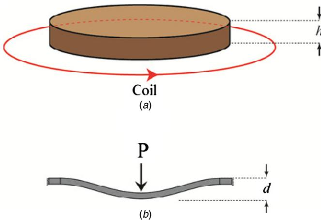
**Figure 2.** Parameters influencing the design of the ferrofluid-based pressure sensor.
