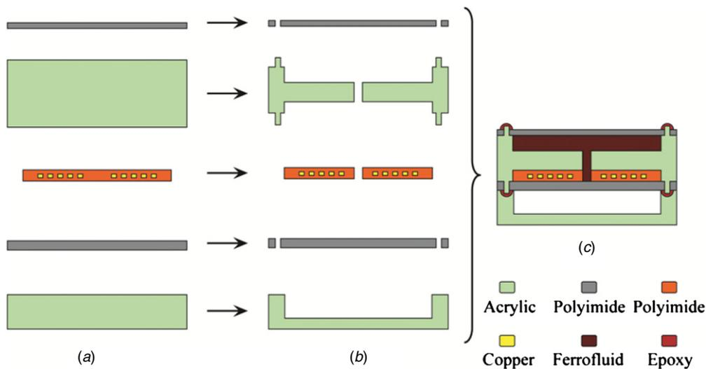
**Figure 4.** Fabrication process of ferrofluid-based pressure sensor.
