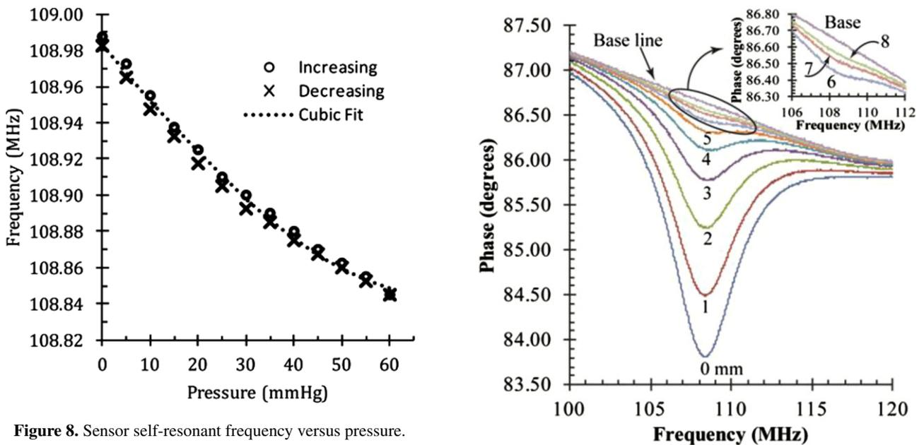
Figure 8. Sensor self-resonant frequency versus pressure.
