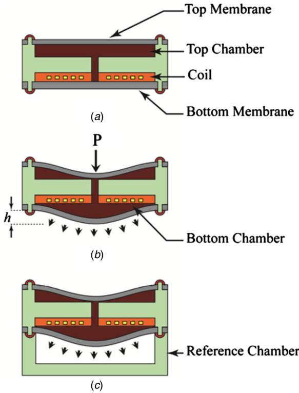
**Figure 1.** Schematic diagram of ferrofluid-based pressure sensor (dimensions not to scale).
