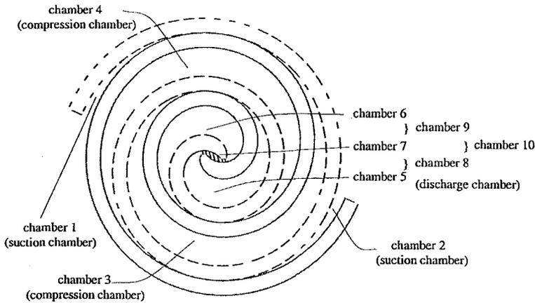
Figure 1. Definition of various compressor chambers
