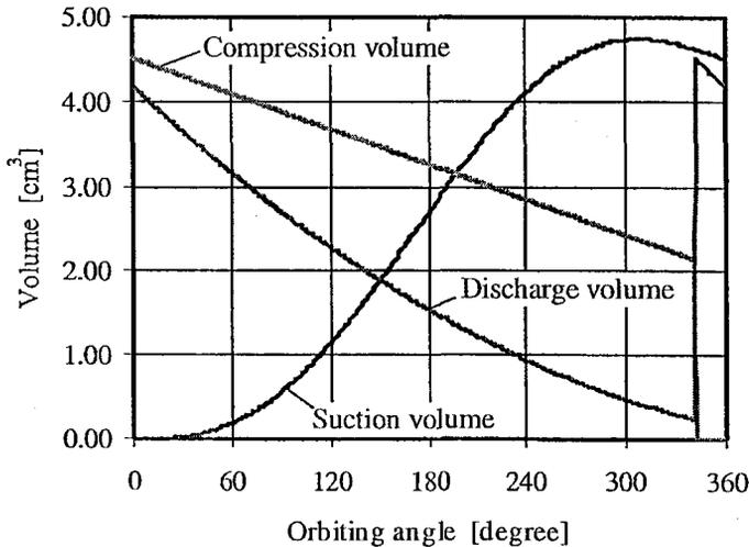
Figure 2 Suction, compression and discharge volume vs. orbiting angle
