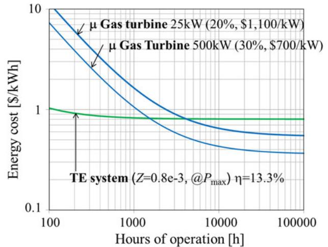
Fig. 3. Energy price versus hours of operation of the generators. The TE system is optimized for maximum power output. The material properties of the thermoelement are thermal conductivity of 4.1 W/mK, electrical conductivity of  $3.7 \times 10^4$  1/Ω m, and Seebeck coefficient of 300 μV/K. The efficiency at maximum power is 13.3%.
