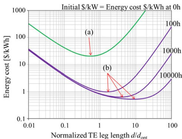
Fig. 5. Energy cost versus hours of operation of the TE generator with variation of element thickness  $d/d_{opt}$ : (a) initial cost (at 0 h), and (b) energy cost at various operation times (100 h, 1000 h, and 10,000 h).
