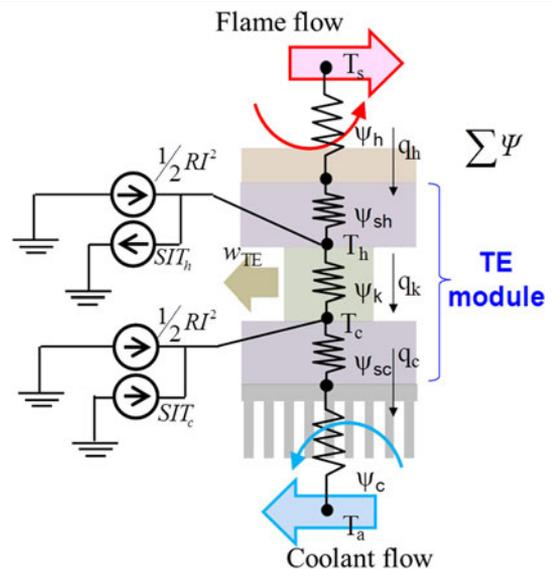
Fig. 2. Diagram of the thermal network of the TE generator system.
