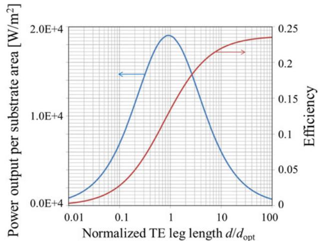
Fig. 4. Power output and efficiency changing only the leg length  $d$  normalized to the optimum leg length  $d_{opt}$ .
