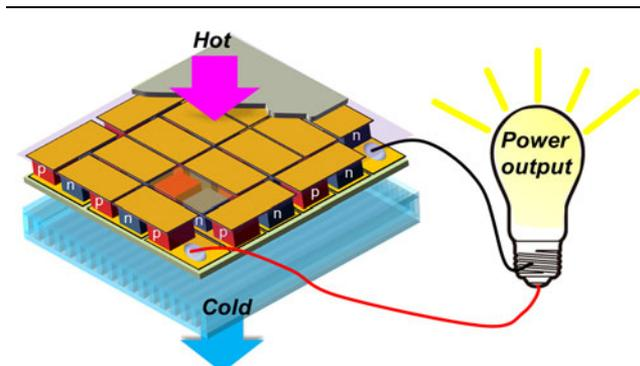
Fig. 1. Conceptual schematic of the modeled TE generator system.
