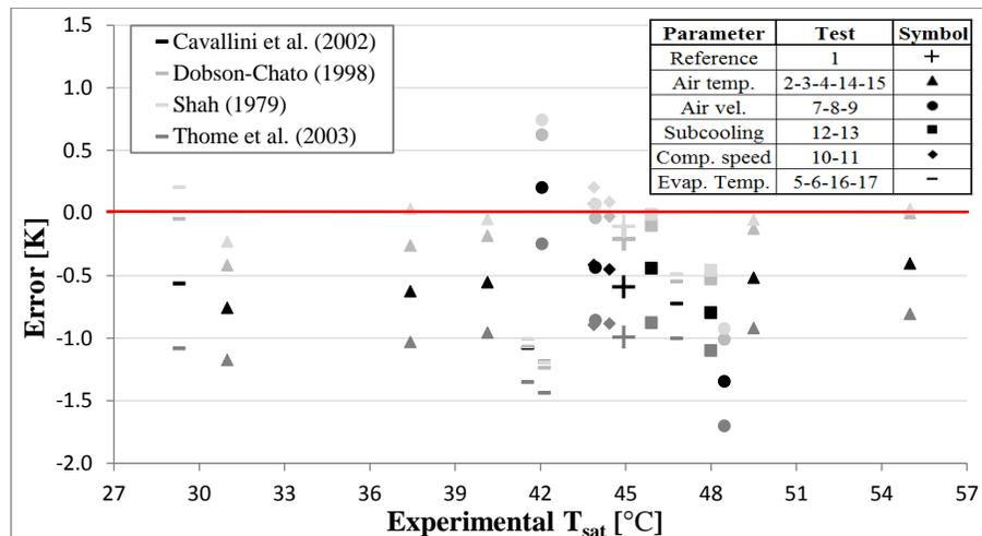
Figure 5: Comparison model plotted versus experimental saturation temperature
