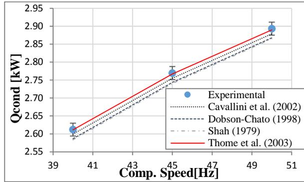
Figure 14: Capacity versus comp. speed
