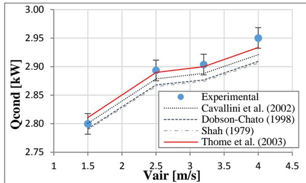
Figure 16: Capacity versus air velocity
