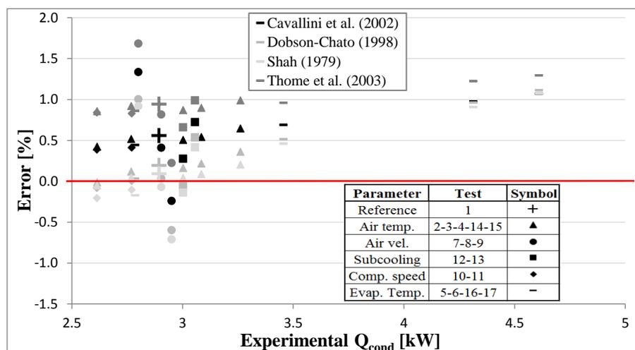
Figure 6: Comparison model versus condenser cooling capacity
