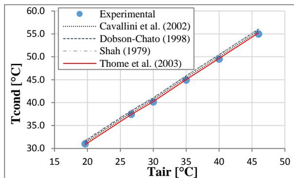
**Figure 9:** Cond. temperature versus Inlet air temperature
