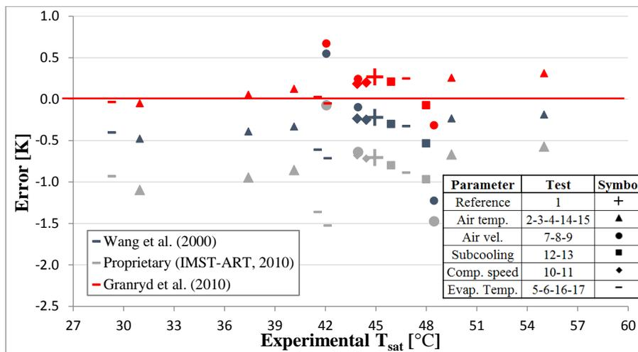
Figure 7: Comparison model plotted versus experimental saturation temperature
