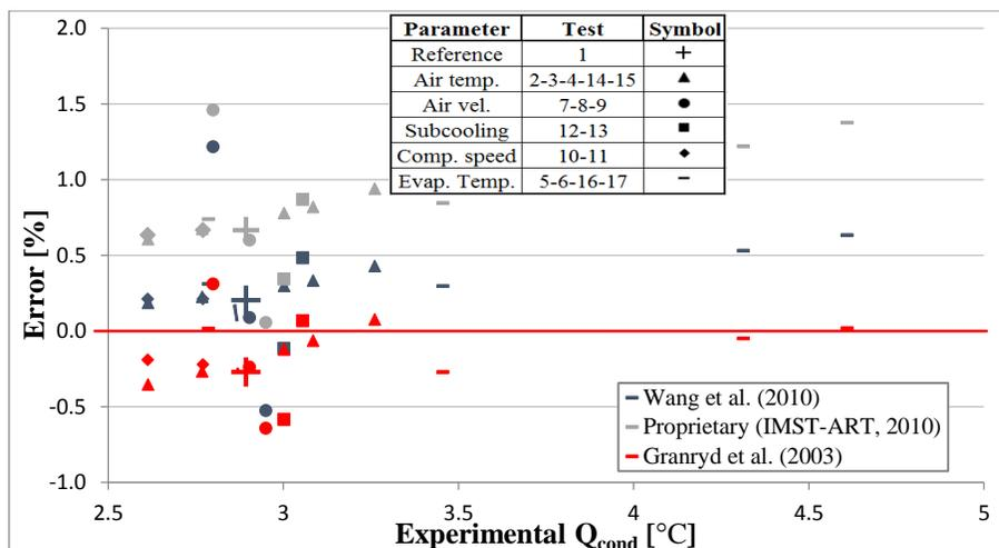
Figure 8: Comparison model versus condenser cooling capacity
