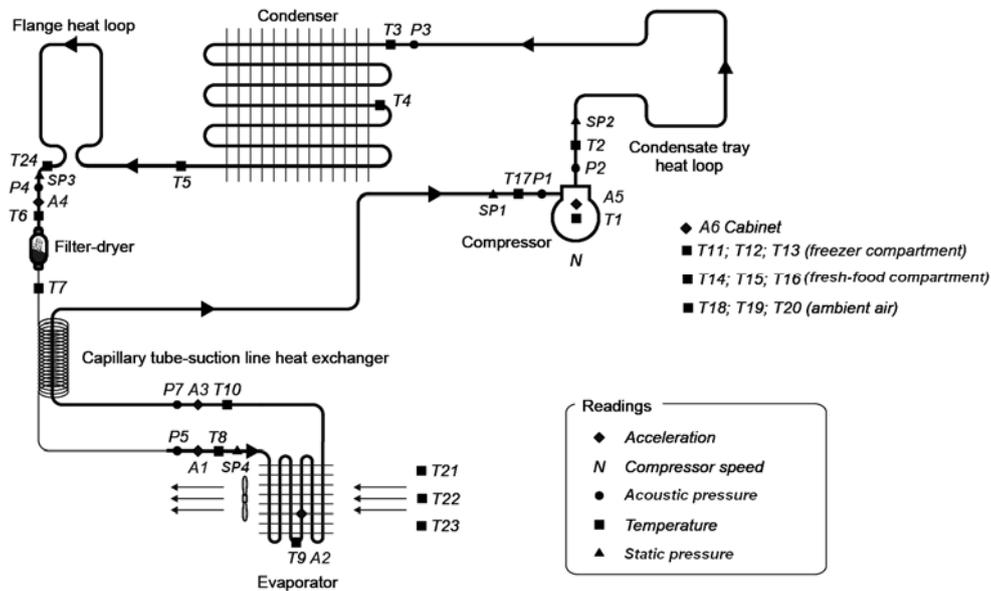
**Figure 2:** Schematic representation of the refrigeration loop
