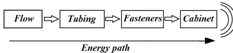
**Figure 1:** Vibratory energy flow in a refrigerator
