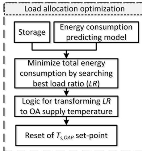
**Figure 4:** Logic of the load allocation optimization module
