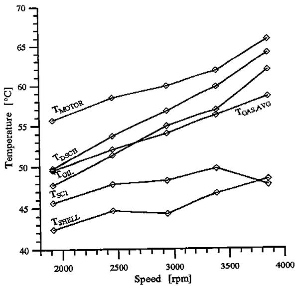
Figure 4: Internal temperatures
