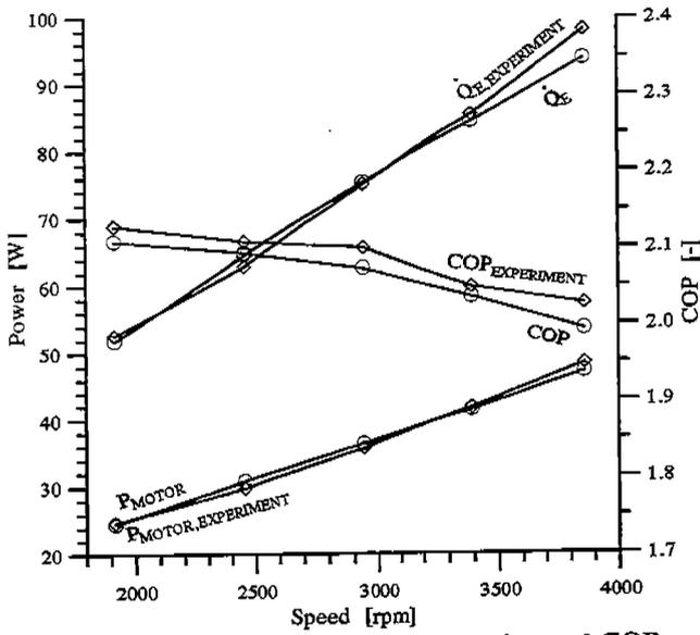
Figure 2: Capacity, power consumption and COP.
