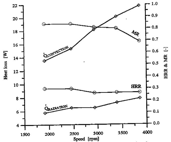
Figure 5: Mixing ratio and shell heat rejection
