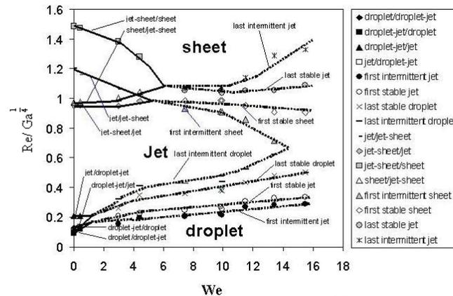
Figure 2: Vapor shear effects on falling-film mode transitions,  $Ga^{1/4}=35.7, s/d=1, s/a=9.3$  (Wei and Jacobi, 2002)
