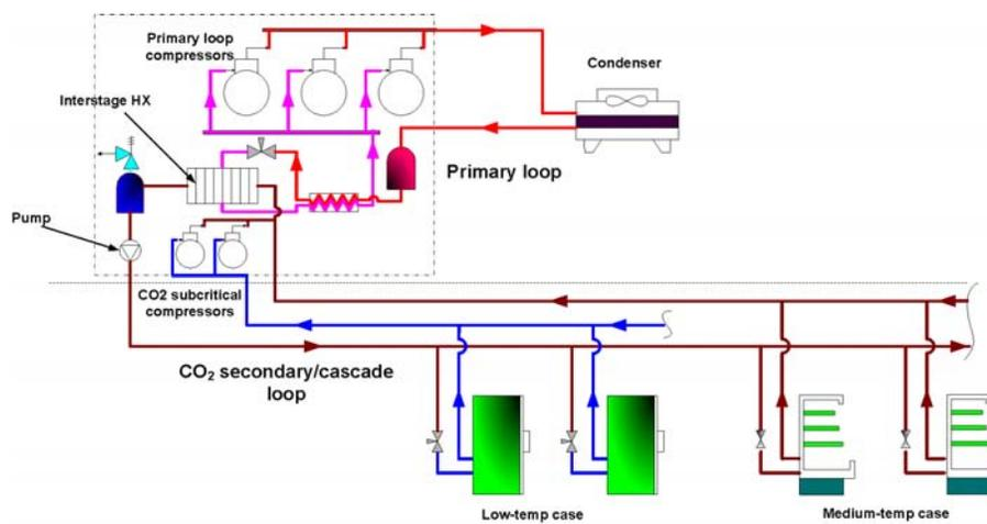
Figure 3: Diagram of CO<sub>2</sub> secondary/cascade system
