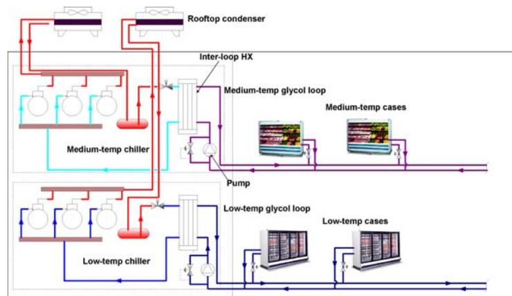
Figure 2: Diagram of single-phase secondary loop system
