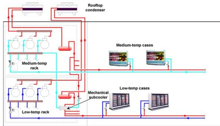
Figure 1: Diagram of parallel rack refrigeration system
