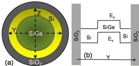
**Fig.1.** (a) Schematic of a circular GAA SiGe/Si core/shell NWFET. (b) Band-edge diagram showing Ec and Ev in the device in the plane of the FET channel.
