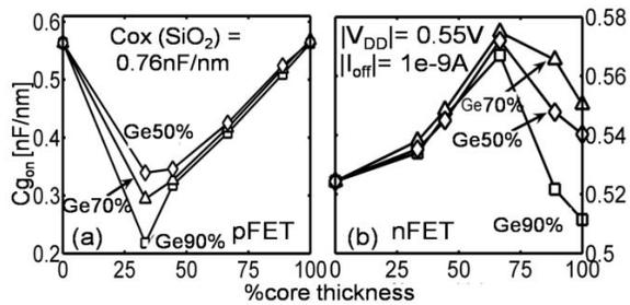
**Fig. 2.** On state gate capacitance (C<sub>gON</sub>) for (a) pFETs and (b) nFETs at V<sub>DD</sub> = 0.5V.
