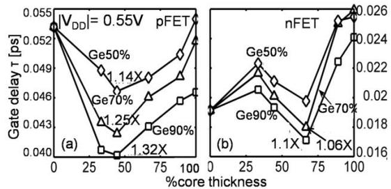
**Fig.4.** Gate delay (τ) for (a) pFET and (b) nFET. SiGe core improves pFETs more (~1.3X) compared to nFETs (~1.1X) over conventional SiNW p/nFETs respectively.
