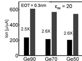
**Fig. 7** pFET improvement (core/shell = 9nm/0nm, tox=1.5nm) using a high-K (HfO) gate dielectric. A 2.5X improvement in Ion is obtained for all Ge%. Thinner EOT brings the charge closer to gate resulting in better transistor action and making I<sub>ON</sub> comparable to nFETs.
