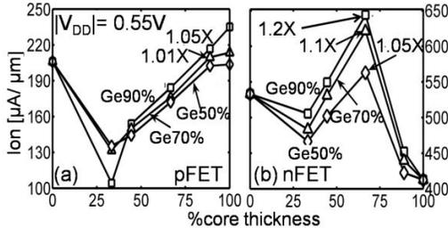
**Fig.3.** Ion for (a) pFET and (b) nFET at V<sub>DD</sub> = 0.55V (normalized to perimeter). Ion increase is monotonic for pFETs. nFETs show highest I<sub>ON</sub> at 75% core thickness
