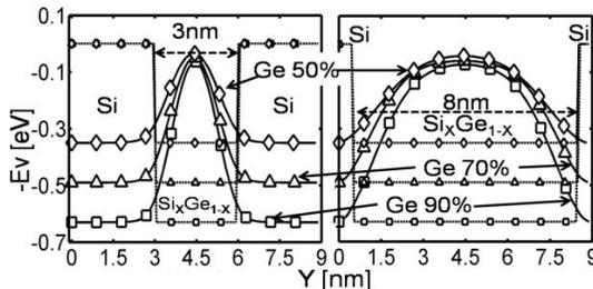
**Fig.5.** Hole cloud under inversion for 3nm and 8nm core for 3 different Ge%. Larger core (thinner shell) brings charge closer to the wire surface thereby improving the pFET.
