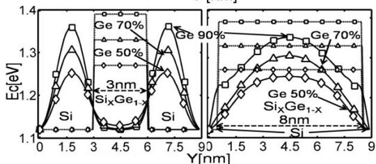
**Fig.6.** Electron cloud under inversion for 3nm and 8nm core for 3 different Ge%. Smaller core pushes the charge closer to wire surface resulting in better nFET performance.
