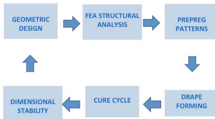
**Figure 2 Carbon fiber prepreg manufacturing simulation**
