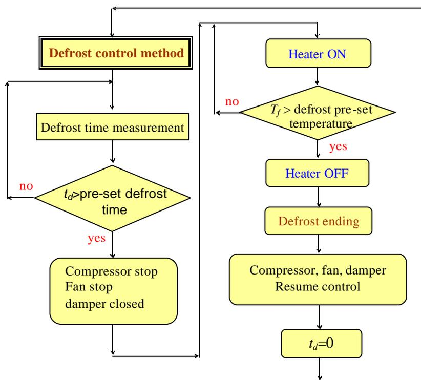
Figure 6: Defrosting Control Method
