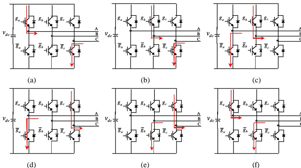
Figure 2: (a)-(f) Control sequence diagram for six-step driving inverter.
