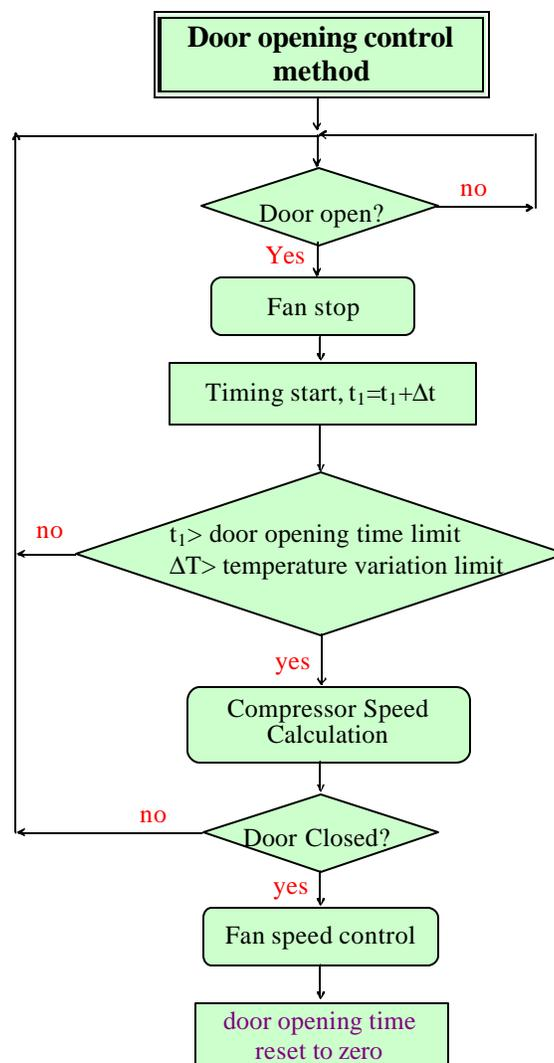
Figure 7: Door Opening Control Method.
