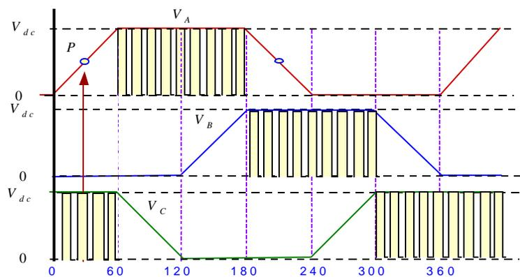
Figure 3: Pulse width modulated voltage waveform.
