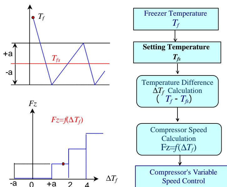
Figure 5: Frozen food storage temperature control flowchart.
