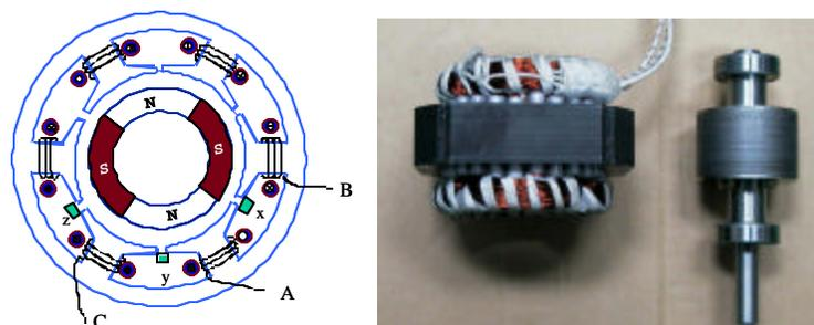
Figure 1: Inner structure and photo of four-pole brush-less DC motor.
