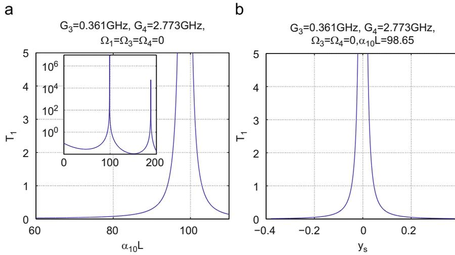
**Fig. 3.** Transmission of the negative-index signal in the vicinity of the higher frequency transition [Fig. 2(a)], controlled by the fully resonant control fields.  $y_s = (\omega_1 - \omega_{ml})/\Gamma_m$ ,  $\omega_2 = \omega_3 + \omega_4 - \omega_1$ .
