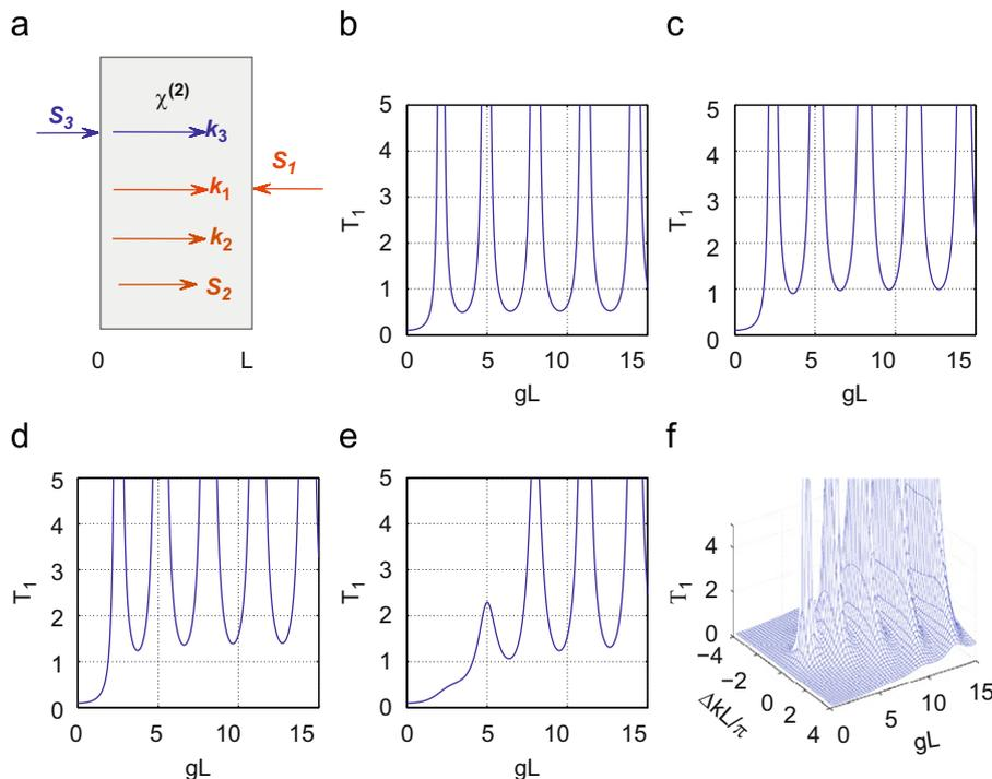
**Fig. 1.** (a) Coupling geometry.  $\mathbf{S}_1$ — negative-index signal,  $\mathbf{S}_3$ — positive-index control field,  $\mathbf{S}_2$ — positive-index idler. (b)–(f) Transmission  $T_1(z=0)$  of the signal at  $\alpha_1 L = 2.3$  and different values of  $\alpha_2 L$  and  $\Delta kL$ . (b)–(d)  $\Delta k = 0$ . (b)  $\alpha_2 L = 1$ ; (c)  $\alpha_2 L = 2.3$ ; (d)–(f)  $\alpha_2 L = 3$ ; (e)  $\Delta kL = \pi$ .
