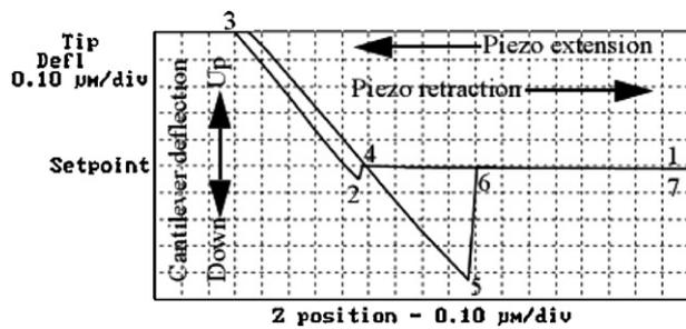
Fig. 1. AFM force curve in contact mode (Digital Instruments, 1996).
