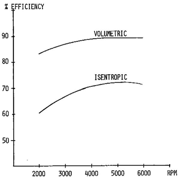
FIG. 10: PERFORMANCE FOR SMALL BOOSTER COMPRESSOR
