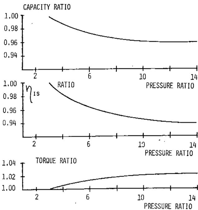
FIG. 1: PERFORMANCE LOSS WITH LIQ. REF. INJECTION
