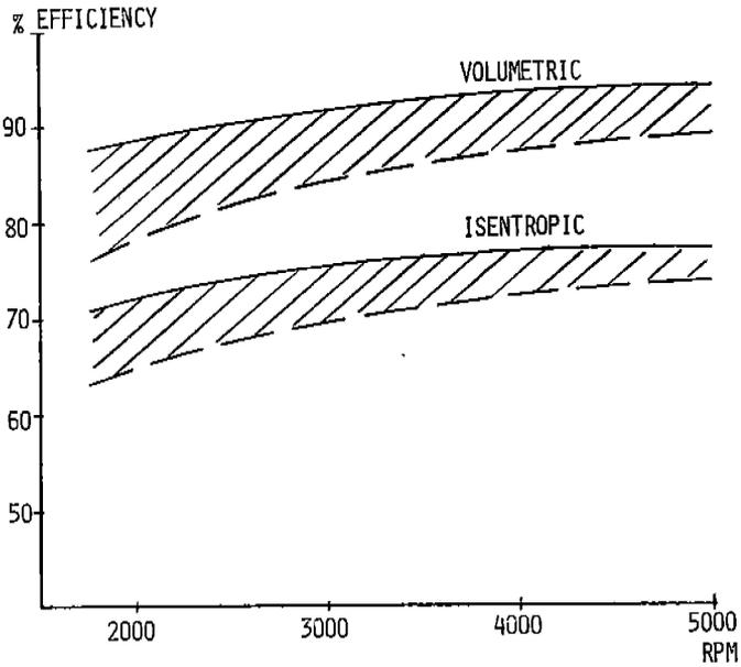
FIG. 8: PERFORMANCE OF TWIN-SCREW COMPRESSOR
