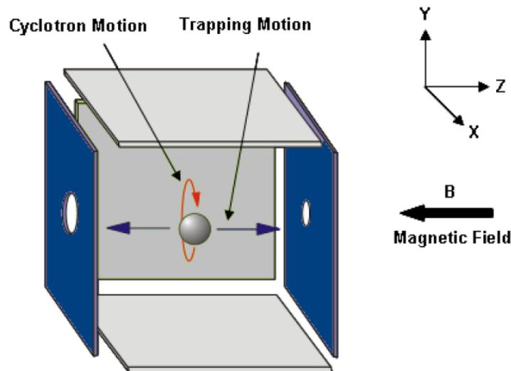
Figure 2.4 Cyclotron and trapping motions of an ion in an ICR cell
