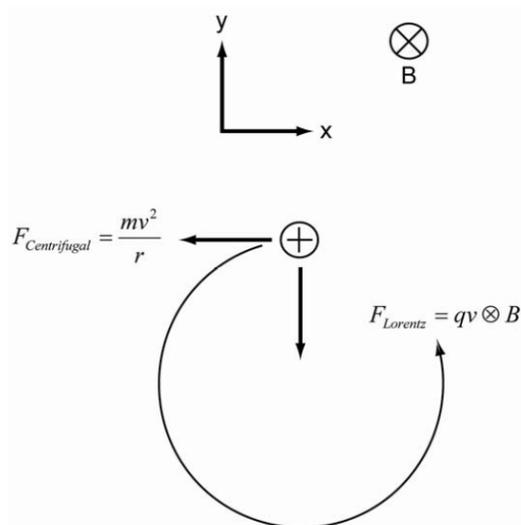
Figure 2.3 The cyclotron motion of a positive ion in the x-y plane perpendicular to the magnetic field
