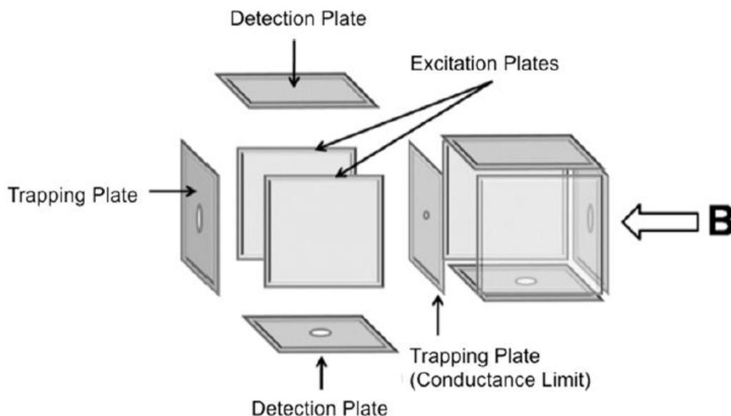
Figure 2.2 The source cell (left) and analyzer cell (right) are divided by the conductance limit. The excitation and detection plates are perpendicular to the magnetic field, and the trapping plates are parallel to the magnetic field
