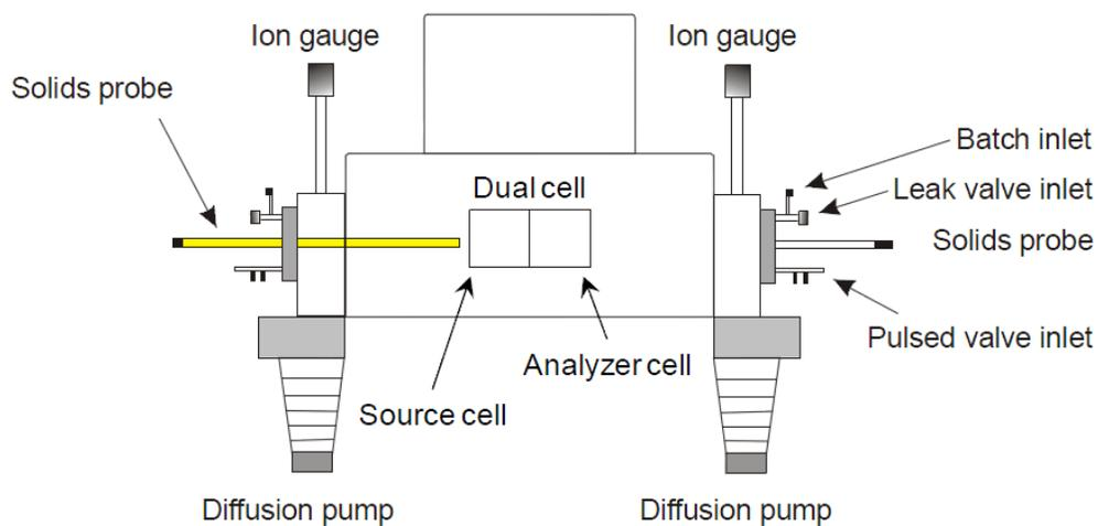
Figure 2.1 Schematic of the dual cell FT-ICR mass spectrometer used in this research
