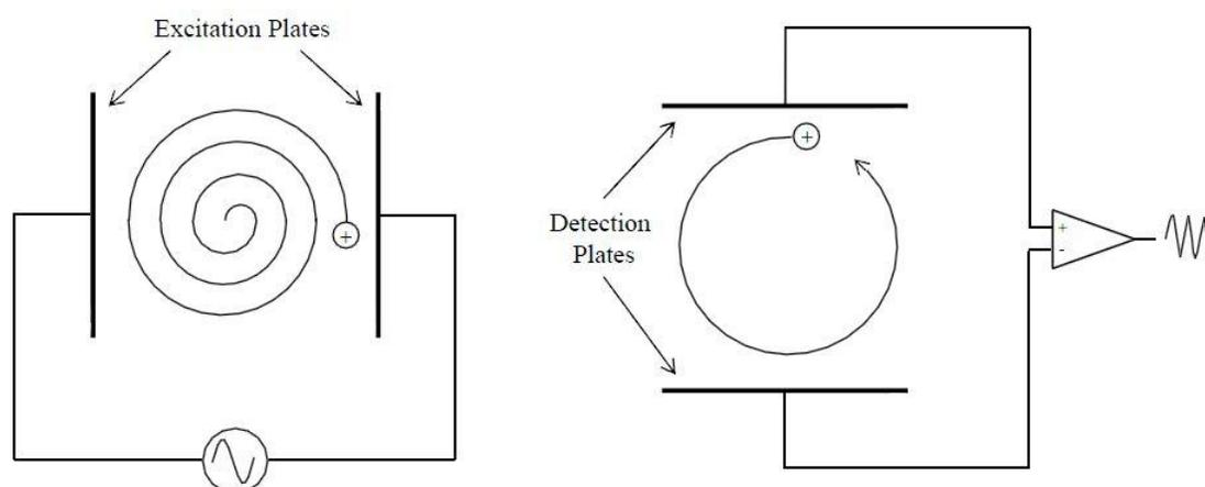
Figure 2.6 Illustration of ion excitation and detection. An rf pulse is applied to the excitation plates to increase the radius of ion cyclotron motion (left, excitation), and the induced image current is detected by the detection plates (right, detection).
