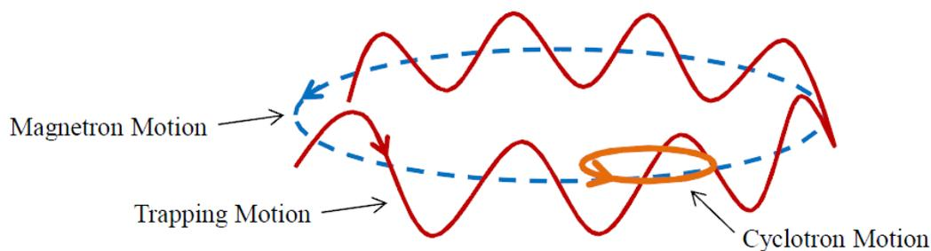
Figure 2.5 All three motions of ions in an ICR cell: cyclotron motion (orange), trapping motion (red), and magnetron motion (blue). The magnetron motion radius is greatly exaggerated comparing to the cyclotron motion in order to show them in the same figure.
