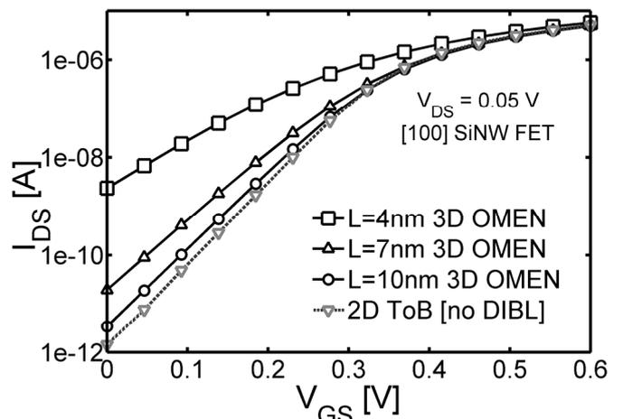
Figure 1.  $I_D$ - $V_G$  plot obtained for a  $3.1 \text{ nm} \times 3.1 \text{ nm}$ , [100] square SiNW with GAA oxide using 3D OMEN for different  $L_c$  and ToB (without DIBL adjustment). At  $L_c=10\text{nm}$ , results from 2 methods are in close agreement.
