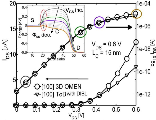
Figure 5. Long  $L_c$   $I_D$ - $V_G$  characteristics for ToB (with DIBL) vs. 3D OMEN for [100] SiNW,  $L_c = 15\text{nm}$ , at  $V_{DS} = 0.6\text{V}$ . Inset shows the variation in the S/D barrier at 4 different  $V_{GS}$  computed using 3D OMEN.  $I_{OFF}$  shows very good agreement; however,  $I_{ON}$  is higher for 3D.
