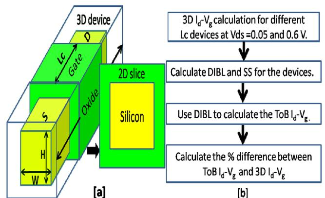
Figure 2. (a) 3D GAA SiNW MOSFET.  $L_c$  shows the gate/channel length. A 2D slice (one unitcell long) from this part is taken for ToB simulation. S and D represent source and drain respectively. W and H are silicon body width and height respectively. (b) Flowchart showing the numerical simulation approach used in this work.
