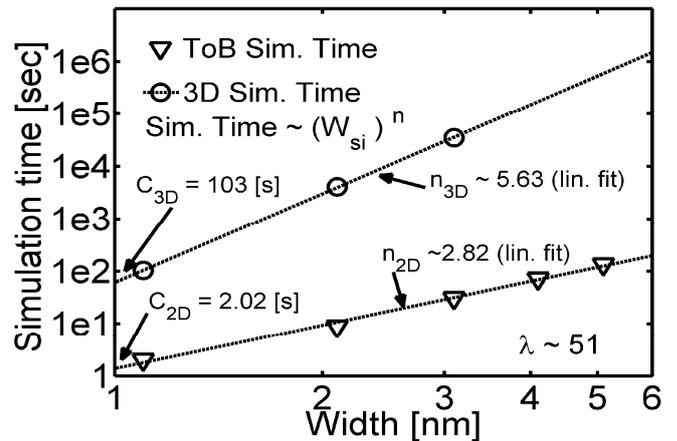
Figure 8. Simulation time for 1 self-consistent iteration for 3D OMEN vs. 2D ToB for a square SiNW with 1nm GAA oxide on 1CPU. ToB simulates  $\sim (W_{si})^2$  times faster compared to 3D OMEN, where  $W_{si}$  is the silicon body thickness.
