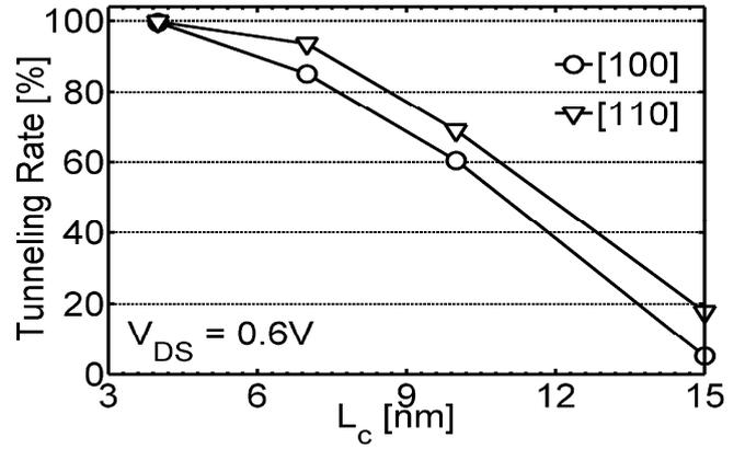
Figure 7. Tunneling current rate percentage in the off-state for [100] & [110] SiNW FETs for different  $L_c$ . Tunneling current decreases in OFF state, as  $L_c$  increases for both [100] and [110]. [110] wires have larger tunneling component hence worse short channel effect (SCE).
