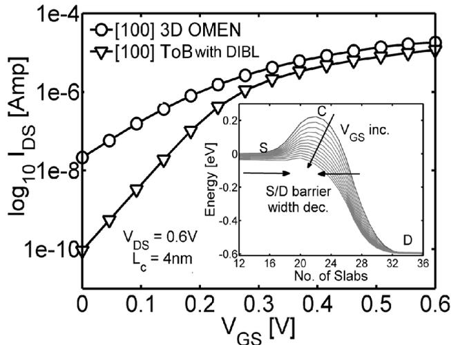
Figure 6. Short  $L_c$  comparison of  $I_D$ - $V_G$  from ToB (with DIBL) with 3D OMEN, for [100] SiNW FET,  $L_c=4\text{nm}$ . Inset shows the S/D barrier for the device which decreases in width and height as  $V_{GS}$  increases.
