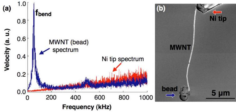
**Figure 3.** In (a), the velocity frequency spectrum of a MWNT showing a vibration peak at 53.3 kHz that is attributed to the bending oscillation of the MWNT. In (b), an SEM micrograph of the MWNT with a gold-coated glass bead affixed to the MWNT tip. The arrows represent where the laser vibrometer was focused on the bead and Ni tip.
