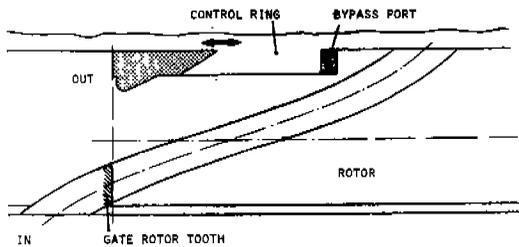
Fig. 29 Capacity control system for Globoid compressors
