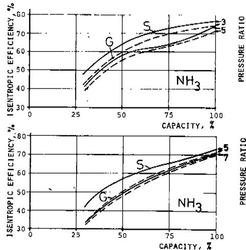
Fig. 33 Ammonia compressor efficiencies at part load for the SRM and the Globoid compressors
