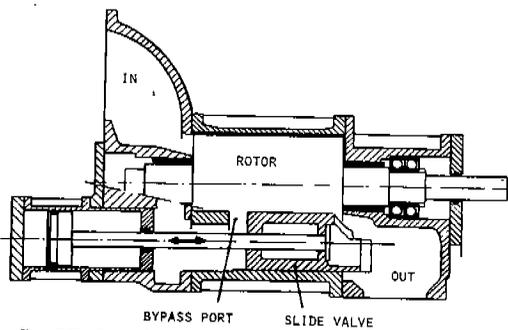
Fig. 27 Capacity control system for SRM compressors
