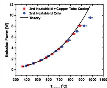
Double heat shield and passive cooling for the waveguide are designed to alleviate the non-idealities in the calibration. The final calibration result shows that the theoretical and experimental data fit well after both corrections.
