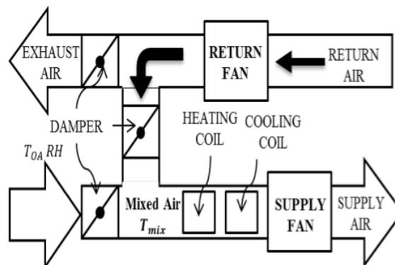
**Figure 1: AHU with airside economizers main components**
