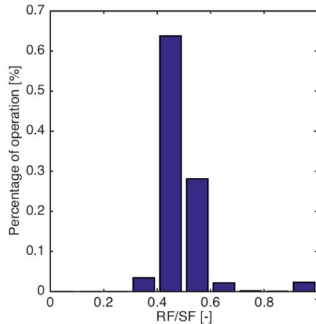
**Figure 6: Frequency of return over supply flow ratio for AHU4 in PHO for Mar-Sep 2014**
