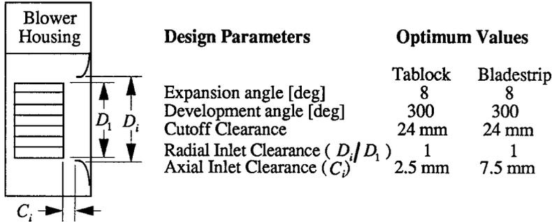
Figure 1. Blower design parameters and their optimum values.
