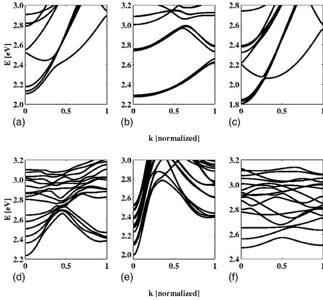
FIG. 3. Conduction subbands of infinite (in the transport direction) nanowires without an applied bias. The cross sections and the crystal orientations are the same as in Fig. 2: (a) Si rectangular wire, (b) Si triangular wire, (c) Si circular wire, (d) GaAs T-shape wire, (e) GaAs hexagonal wire, and (f) GaAs rectangular wire.
