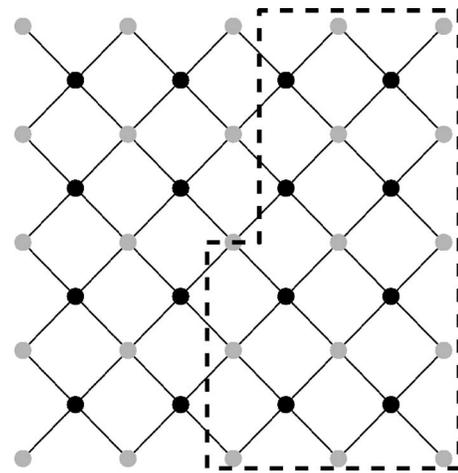
FIG. 10. Cross section of a rectangular GaAs wire with rotational symmetry properties around its center.
