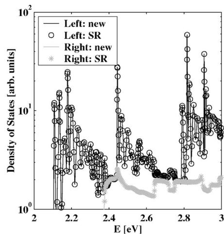
FIG. 6. Electron density of states (DOS) for the same wire and the same conditions as in Fig. 5. The results obtained with the present method (lines) are compared to the results from the Sancho-Rubio iterative algorithm (Ref. 15) (symbols): the contribution to the total DOS coming from the left contact (dark line and circles) and coming from the right contact (light line and stars) are shown in the first device slab ( $0 \leq x \leq 0.543$  nm).
