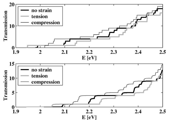
FIG. 8. Electron transmission for the GaAs hexagonal wire in Fig. 2 without strain (dark solid line), with a biaxial tension  $\epsilon_{yy}=\epsilon_{zz}=0.015$ ,  $\epsilon_{xx}=-0.0087$  (light solid line), and for a biaxial compression  $\epsilon_{yy}=\epsilon_{zz}=-0.015$ ,  $\epsilon_{xx}=0.0087$  (dark thin line). (Up) no bias. (Down) bias of 0.1 V.
