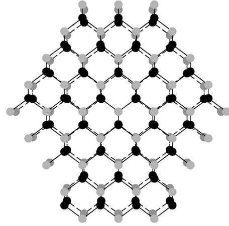
FIG. 7. Superposition of an unstrained (dashed atom connections) and of a strained (solid atom connections) GaAs hexagonal wire cross section. The unstrained case corresponds to wire (e) in Fig. 2. An homogeneous biaxial tension is applied in the strain case ( $\epsilon_{yy}=\epsilon_{zz}>0$ ).
