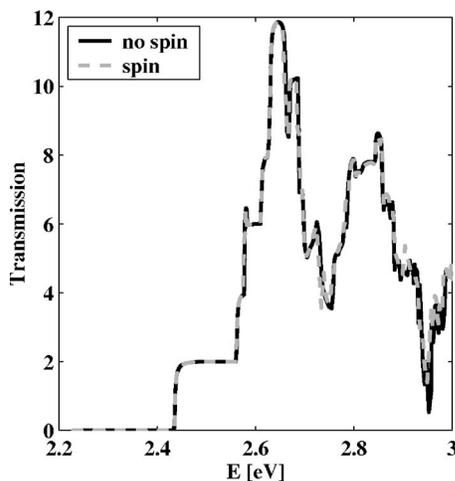
FIG. 9. Electron transmission through the GaAs T-shape wire in Fig. 2 for an applied bias of 0.2 V, calculated with (light dashed line) and without (dark solid line) spin orbit coupling.
