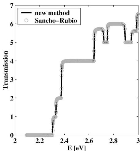
FIG. 5. Electron transmission through the Si rectangular [100]-oriented wire in Fig. 2 for an applied bias of 0.2 V. The results obtained with the OBC method presented in this paper (solid line) are compared to the results from the iterative algorithm proposed by Sancho and Rubio (Ref. 15) (bright circles).
