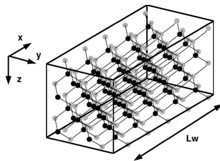
FIG. 1. Schematic view of an atomistic nanowire.  $x$  is the transport axis,  $y$  and  $z$  are confinement directions,  $L_w$  represents the wire length. Each atom is considered as well as the connections to its four nearest neighbors, except at the surface.
