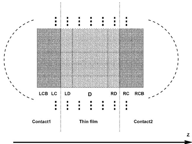
**Fig. 1 Schematic diagram of a five-unit-cell thin film between two semi-infinite contacts. The definitions of different groups of atoms are shown. In this case, Region D includes three unit-cell layers.**
