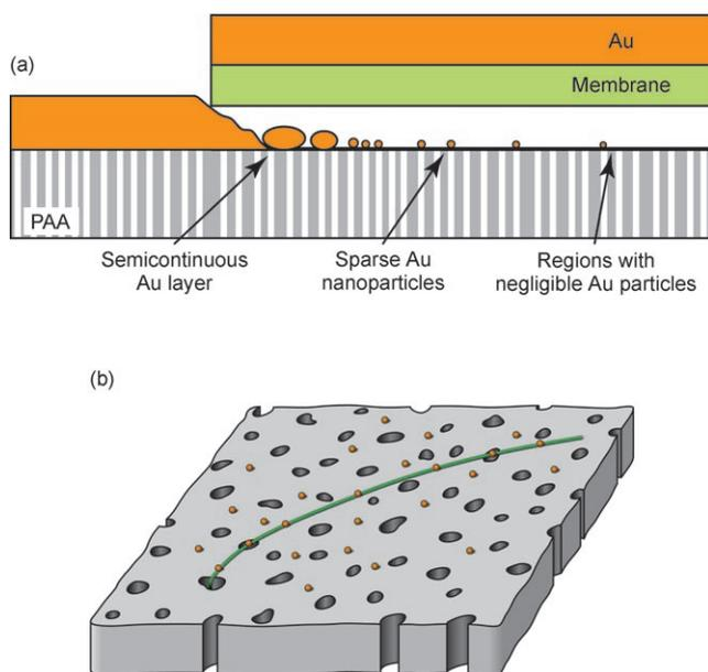
**Figure 2.** a) Schematic representation of the three regions with different Au particle distribution on the PAA film after Au evaporation through a nitride membrane mask. b) Enlarged view of region (ii), showing one CNT emerging from a pore and growing along the PAA surface. Au nanoparticles diffuse into this region and attach to the CNT.
