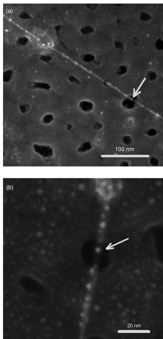
**Figure 4.** Sub-5-nm gold nanoparticles suspended on the CNTs. a) Sub-5-nm gold nanoparticle indicated by white arrow is on a CNT and above the pore in the PAA film. b) 3-nm gold nanoparticle suspended on a pore by the CNT. This image is from an area with a 10- $\mu$ m gap with more available gold nanoparticles migrating from the large gold pads.
