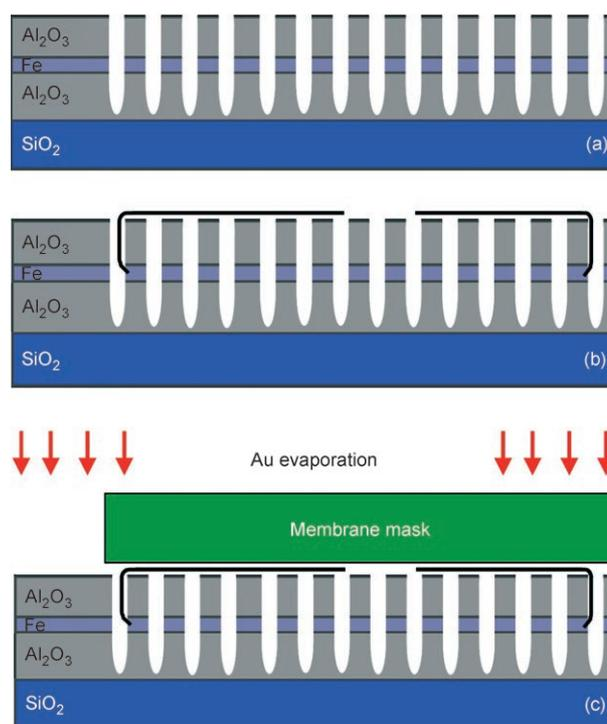
**Figure 1.** a) Diagram of a cross section of a PAA film with an iron layer as catalyst. The pores are formed by anodization of the Al film, which also anodizes through the Fe layer. b) SWNTs are grown from these pores by PECVD. c) A membrane mask is used during evaporation to pattern a Au film.
