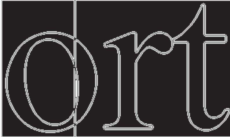
Figure 1. The edge map of an image. Black pixels represents non-trappable pixels, white pixels represents edge2 pixels, and gray pixels represents edge1 pixels.
