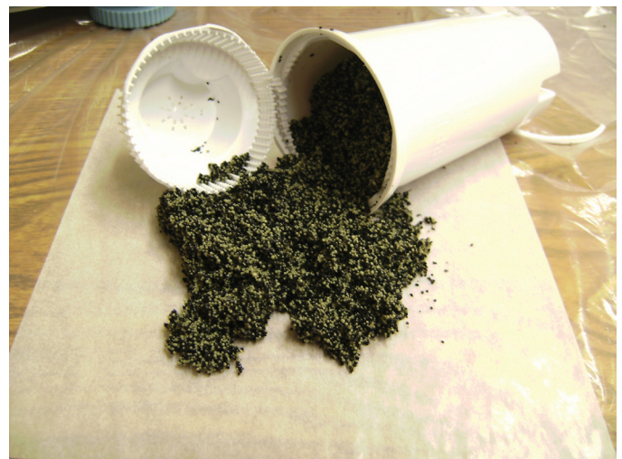
Anionic resin and activated carbon, the heart of the pitcher water filter.
