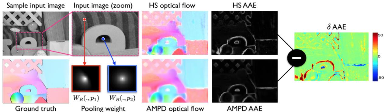
Figure 1: Sample results using sequence "RubberWhale" from Middlebury training set. Optical flow are represented using the color from [1]. We show how pooling weight are adaptive depending on position and comparisons of optical flow between HS and APMD with Average Angular Error (AAE).
