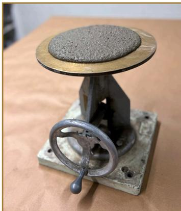
Mortar flow table testing was used to characterize SAP's effect on flow. Here, a 0.42 w/c mortar containing SAP and 0.5% HRWRA flowed 93%.
