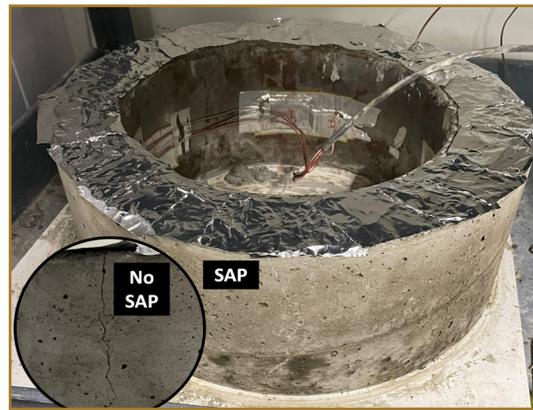
Ring testing of cracking tendency under restrained shrinkage. The 0.35 w/c Type I mortar with SAP ring is uncracked, while the inset shows a 0.35 w/c Type I mortar of the same age which has cracked.
