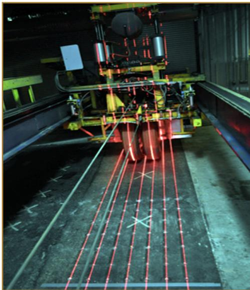
Accelerated pavement testing (APT) machine.
