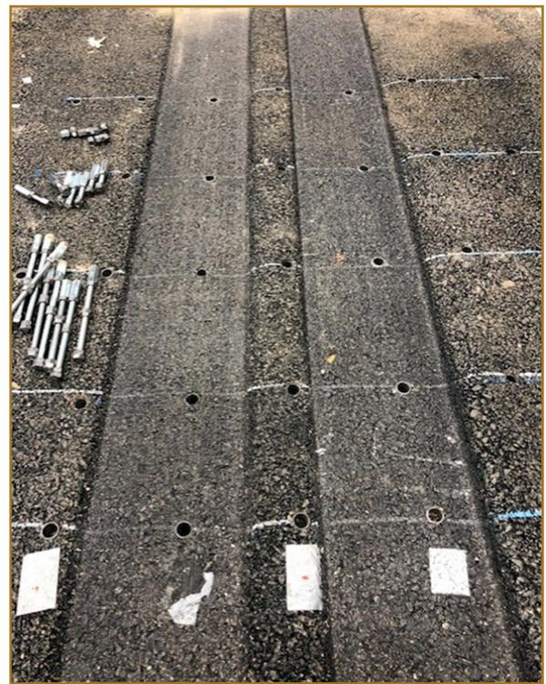
Fabricated holes to monitor the layer deformation.
