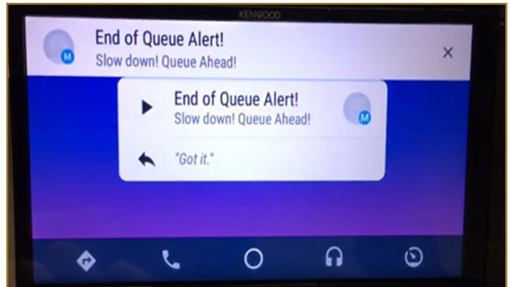
The alert messages will be sent through Android-based smartphone apps via the 4G network and the Android Auto device.
