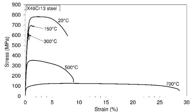
Figure 3 Engineering stress-strain diagrams at different temperatures: X46Cr13 steel.
