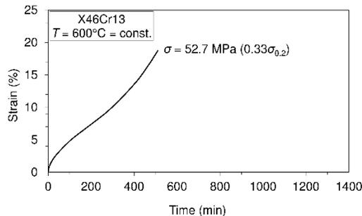
**Figure 5** Short-time creep behavior of steel X46Cr13 at the temperature of 600°C.
