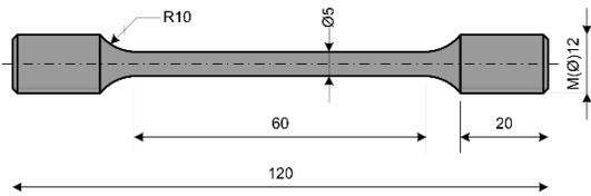
Figure 1 Specimen used in tensile tests, geometry (mm).
