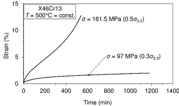
**Figure 4** Short-time creep behavior of steel X46Cr13 at the temperature of 500°C.
