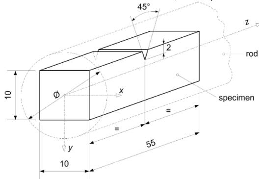
Figure 2 Charpy V-notch specimen (mm).
