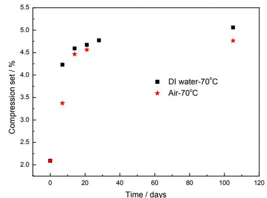
**Figure 2** Compression set of aged silicone rubbers with or without DI water
