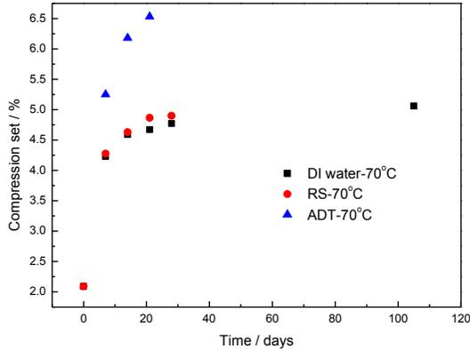
**Figure 3** Compression set of aged silicone rubbers in different test solutions
