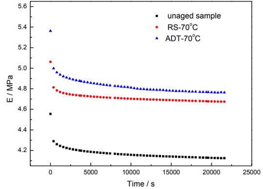
**Figure 5** Time dependent compression stress relaxation modulus E of silicone rubber exposed to test solutions at the temperature of 70 °C
