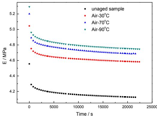
**Figure 4** Time dependent compression stress relaxation modulus E of silicone rubber at three different temperature levels
