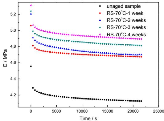
**Figure 6** Time dependent compression stress relaxation modulus E of silicone rubber exposed to RS up to 4 weeks at the temperature of 70 °C
