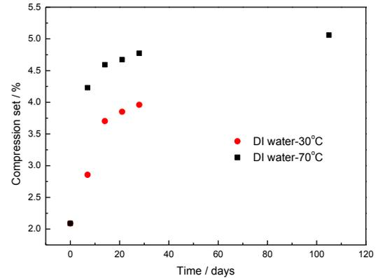
**Figure 1** Compression set of silicone rubbers exposed to DI water at 30 °C and 70 °C
