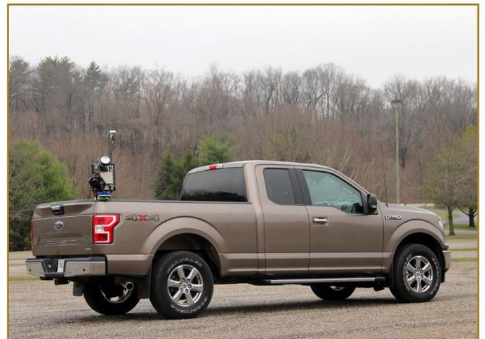
*The portable Backpack system mounted on a carrier vehicle.*
