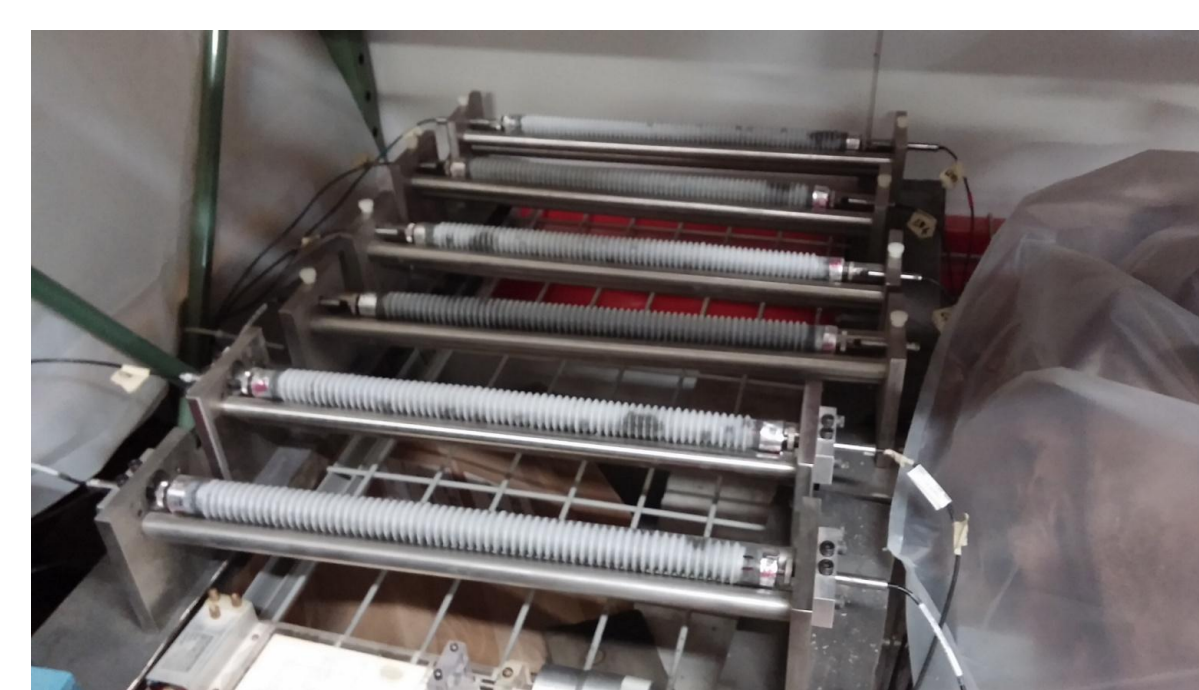
Figure 3: A row of mortars undergoing autogenous shrinkage
