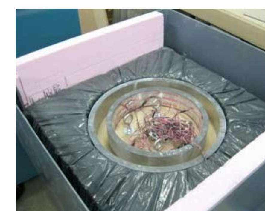
Figure 4: Dual Ring Apparatus in insulation chamber, Reference: J. L. Schlitter et. al.
